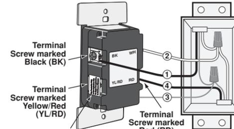
**Terminal Label:** Use terminal for 3-way or more applications only. For single-pole applications, DO NOT remove label.
